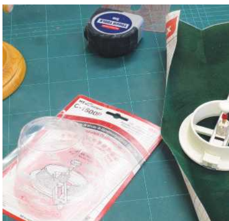
▲ Pic.34 Once it's all glued together you can put baize on the bottom. This is Les's new circle cutter, the benefit of which is that it doesn't make a hole in the middle
